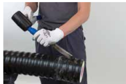
(3) Split the casing pipe with a knife or chisel. Note: Ensure you don't damage the service pipe.
