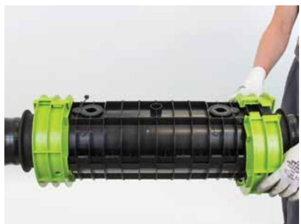
(6) Secure the sealing ring into place by installing the two halves of the green clamps.
