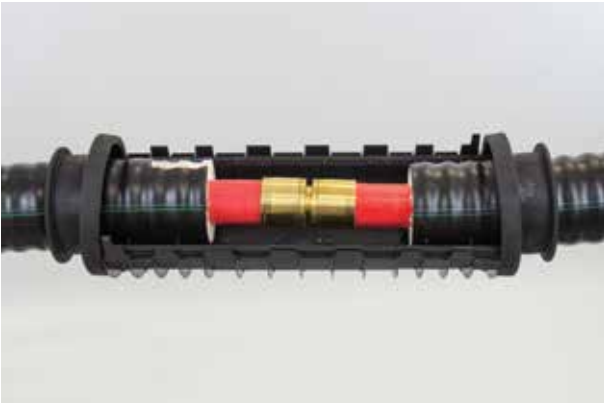
(1) Position the lower shell sleeve so that its edges fit inside the sealing rings. Note that the lower half of the shell sleeve does not have any plug holes.
