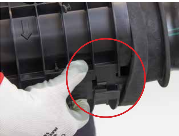
(3) Move the two halves of the shell joint together and allow the longer catches to click into place (see photograph).
