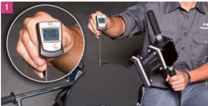
Measurement of temperature at the butt-welding machine
